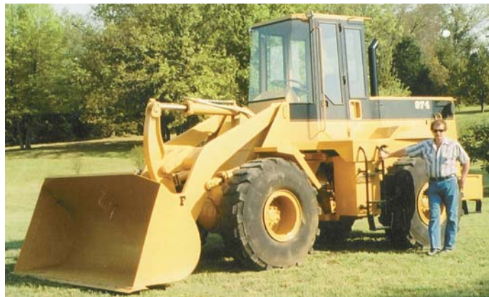
Stephen Foster built this loader from scratch for only about $5,000, patterning it after a Caterpillar 950.
