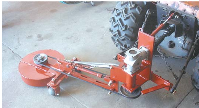
Home-built, 3-pt. mounted mower reaches under low lying fence lines, automatically gliding around posts. A right angle gearbox belt-drives a pulley mounted on top of deck.
