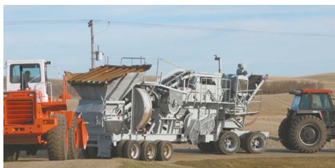
After purchasing this 1949 rock crusher, Wayne Hagen added a tandem axle and hitch on front so he can pull the 60,000-lb. machine with a tractor.
