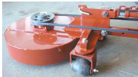
Home-built, 3-pt. mounted mower reaches under low lying fence lines, automatically gliding around posts. A right angle gearbox belt-drives a pulley mounted on top of deck.
