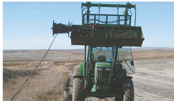
Hydraulic-powered wire winder bolts to side of Gutschmidt's loader bucket.
