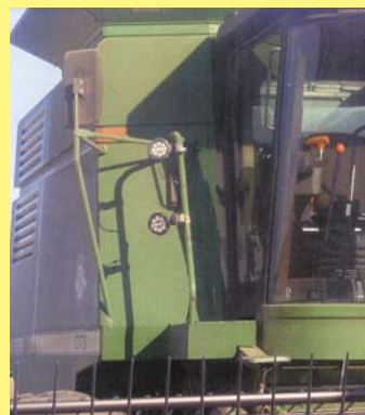
LED work lights are brighter, last longer and consume less power than standard halogen lights, according to Hamsar.
