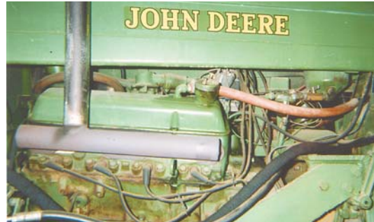
"Mounting a 307 Chevy V-8 engine in my Deere G was a lot of work, but it was worth it," says Howard Harder.
