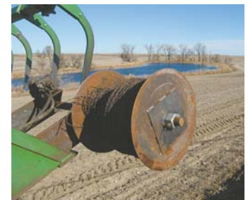
Wire winder consists of a main shaft, bearings, disc blades, and a hydraulic motor.
