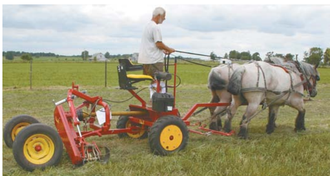
Carts can be ordered with rubber or steel wheels, optional brakes, and either a cast aluminum or cushioned seat.
