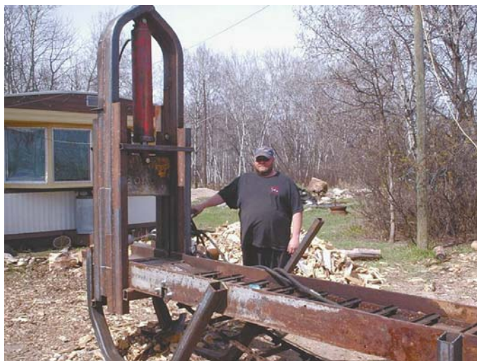
Double-edged blade on firewood "guillotine" slices through whole trees, cutting them into 6-in. lengths and splitting them at the same time.
