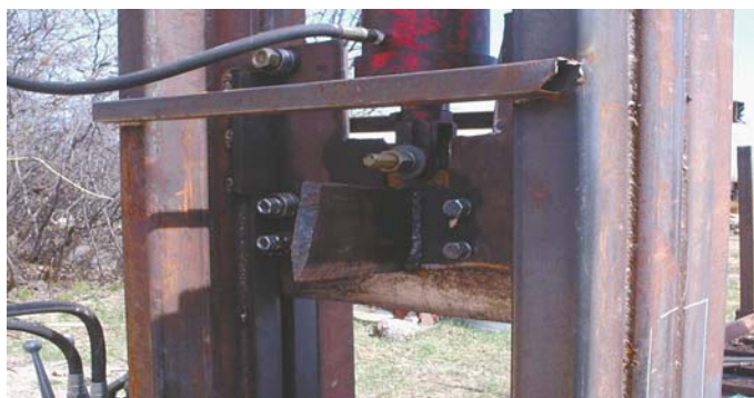
Guillotine's 22-in. wide by 16-in. high cutting blade was salvaged from a Caterpillar dozer blade.
