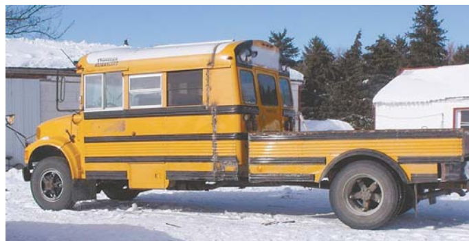
Fred Callens converted a 1990 IH 77-passenger bus into a giant yellow pickup. "It does the work of 1-ton duals that costs $40,000 or more," he says.
