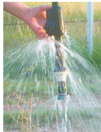
Filter fits between the hose and the regulator on center pivot drop nozzles (left). To flush out sediment you just push up a small release valve on side of filter.
