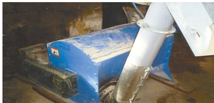
Rotary mill is belt-driven off a 10 hp electric motor and has no rollers, hammers or screens (above). Instead, it uses a high rpm open cylinder set inside a drum. Cylinder is equipped with 6 welded-on, staggered shear bars that pulverize the corn.
