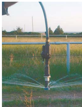
Filter fits between the hose and the regulator on center pivot drop nozzles (left). To flush out sediment you just push up a small release valve on side of filter.
