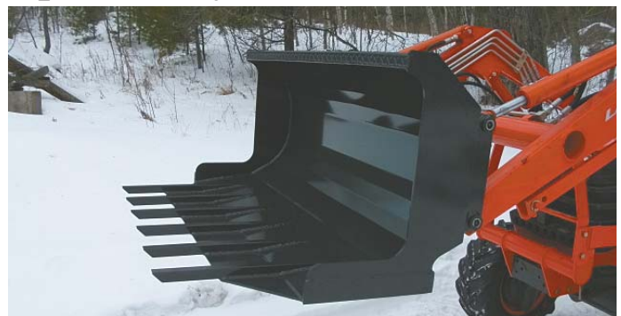
Jery Dunn's Loader Buddy has 6 tines that extend 5 in. beyond bucket's lip. Note cut-out end plates.
