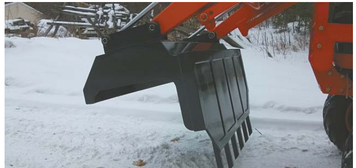
With bucket rolled all the way forward, tines point back toward tractor making it easy to loosen ground while backing.
