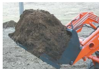
Even with cut-out end plates, bucket can hold a lot because its bottom plate extends 4 in. farther forward than on a conventional bucket (above). Cut-out end plates allow bucket to handle logs (below). Bucket teeth can also be used to dig rocks and tree roots, as shown at right.
