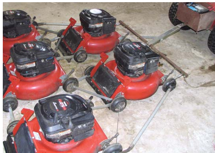
Patrick Roderick built a hitch to pull 5 mower decks behind his 11 hp garden tractor. The 5 mowers cut a 78-in. wide swath.
