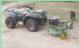
Front-mounted mower (above) mounts to ATV on two ball hitches, allowing mower to maneuver without being too rigid.
