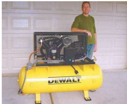
To save money, Eugene Schwanbeck built his own air compressor equipped with a 220-volt, 5 hp electric motor.
