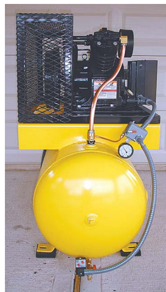
Compressor’s 2-stage pump is driven by a 5 hp single phase, 220-volt electric motor.
