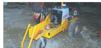
Tom Chaney converted an old Roper riding mower into a “high wheeled” towable welding cart.
