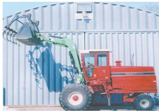
William Leiser's sons convinced their dad to help them build this loader tractor out of a 1980 IH 1460 combine. It's equipped with a Buhler 2795 loader with grapple fork.
