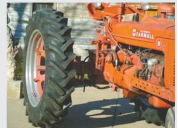
Old-style tires with 45 degree lugs for antique tractors are available from Dawson Tire Service.
