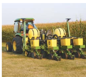
Planter's precision system includes row-by-row shutoffs that can be set and controlled by pre-loaded field maps.
