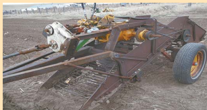
This ground-driven potato digger was given new life by adding hydrostatic drive.
