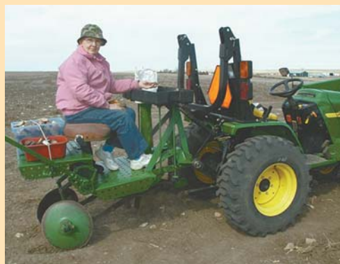
Willard Kanning retooled a used 1-row planter, installing platforms for a helper's seat and to hold extra seed potatoes.
