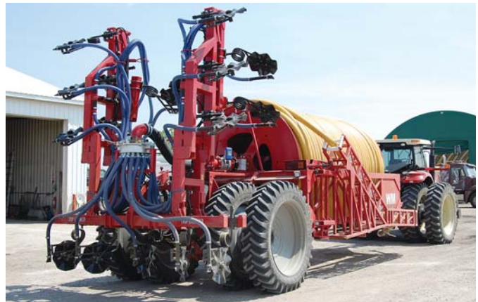
Manders Dairy sidedresses liquid manure in standing row crops using their home-built, 16-row Crop Enhancer applicator.
