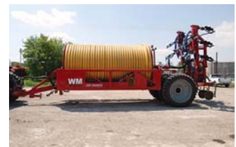
Unit’s 45-ft. toolbar folds to a transport width of 12 ft. Hose wraps around tank.
