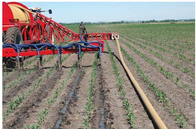
Machine feeds out drag hose as it applies manure between rows.
