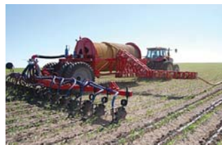
Unit’s 45-ft. toolbar folds to a transport width of 12 ft. Hose wraps around tank.
