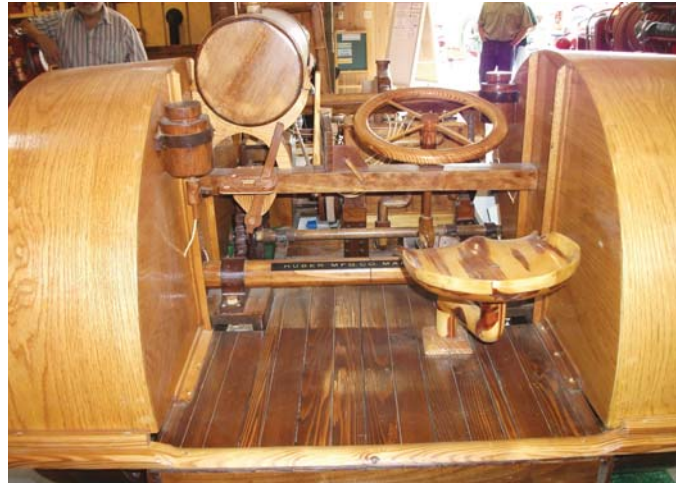
Mike Pray carved this 1/2-scale Huber tractor in wood, recreating individual components and then bolting them together with wooden nuts and bolts.
