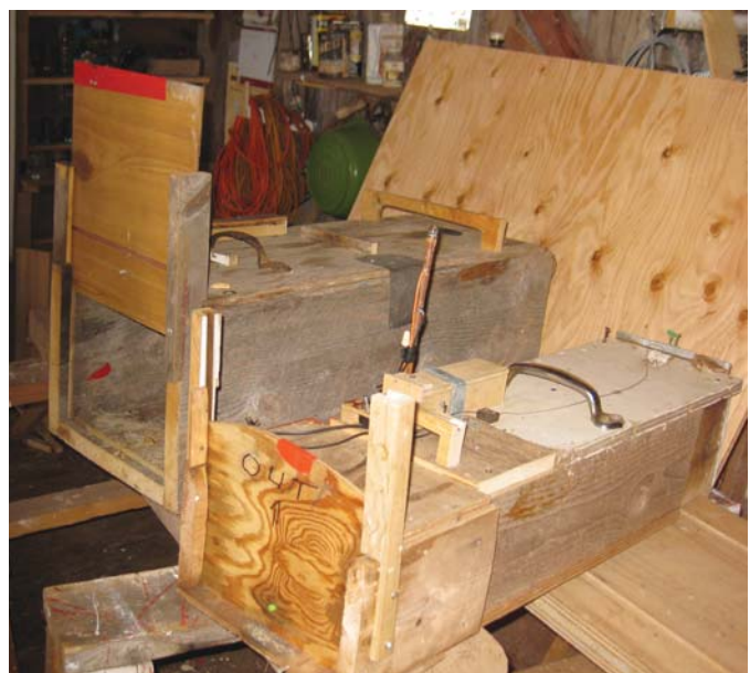
Baited ramp activates a wire that releases a door to fall down when animal is caught, which causes a light to come on.
