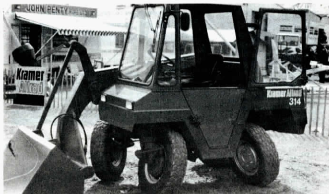
Amazing new German skid-steer loader features sideways movement, plus side-opening cab and one-arm loader.
