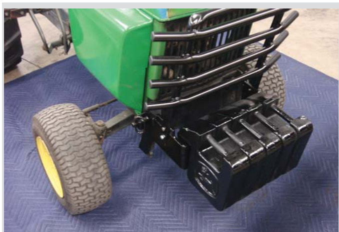
Cargo Gard bracket protects front of tractor. It also holds suitcase weights.
