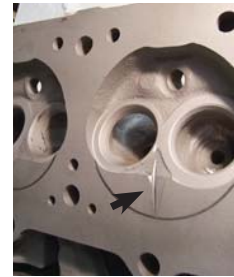
Grooved cylinder heads are said to boost power and result in better fuel efficiency.
