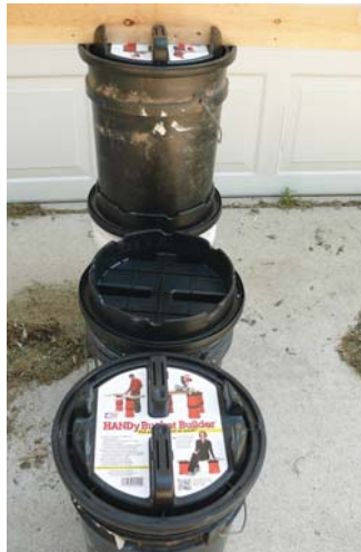
Hard plastic tops fit any standard 5-gal. bucket and, along with 2 by 4 studs, can be used to set up a work bench instantly.
