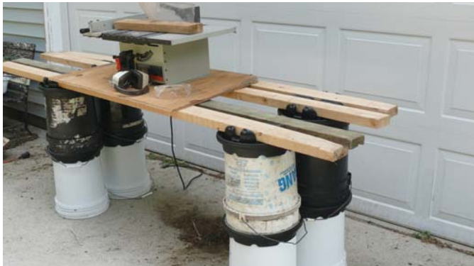
Tabs in the molded plastic tops hold 2 by 4's in place.
