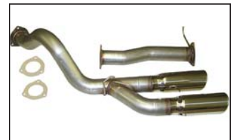
High-flow exhaust kits can improve horsepower output on diesel trucks or simply change their sound or look.
