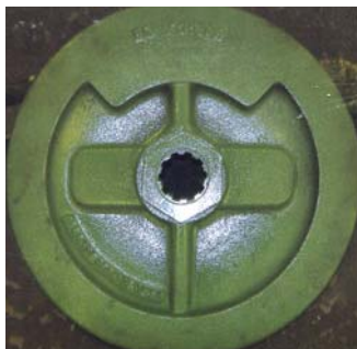
Dave Darr casts new flywheels for 720 and 730 diesels. He rebuilds other models using his Taper-Loc Hub.
