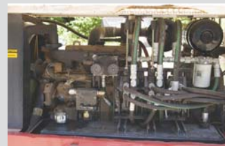
Paul Bedard bought a big Chicago compressor complete with trailer and installed a hydraulic system on it so he has both hydraulic and air power.
