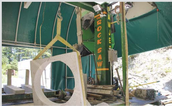
Paul Bedard builds all his own cutting and drilling equipment. This rock saw allows him to slice through 5-ton, 4 by 4 by 8-ft. rocks with ease.
