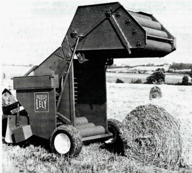
New Lely baler has rollers at the bottom, and adjustable chains and slats at the top.
