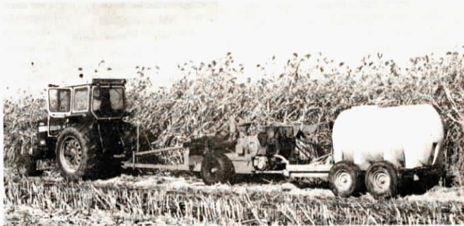
First-of-its-kind machine harvests up to 30,000 lbs. of sorghum juice per acre.
