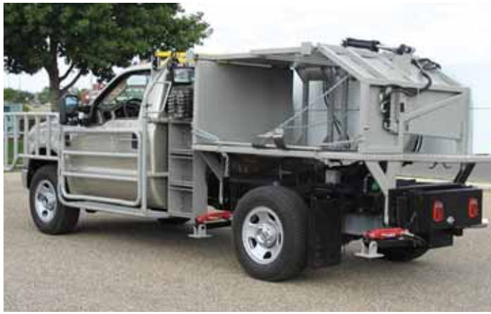
Truck-mounted hoof trimming chute picks the cow up and lays her over in one smooth, fast motion.
