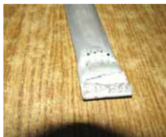
There's a garden hose hook-up at one end of wand and a "pinched down" fan head at the other end. The wand is small enough to fit into tight spots behind radiator.
