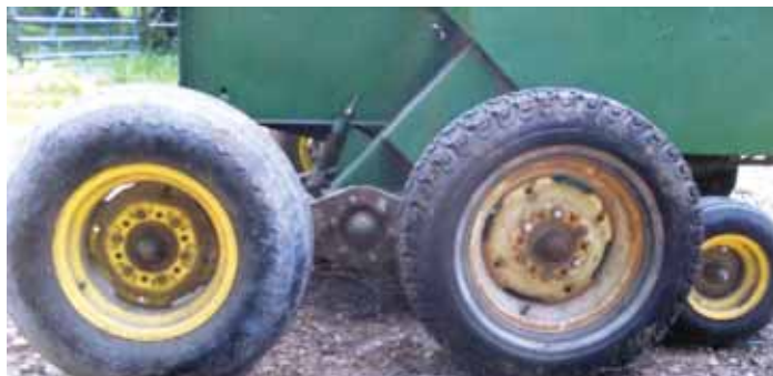
Chad Travis added a walking beam tandem axle to his Deere round baler. "It results in a more even ride that keeps the pickup reel from digging into the dirt," he says.
