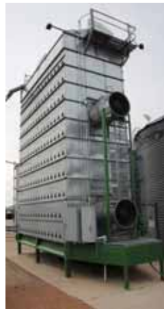
Kelly's dryer has 3 custom-built chambers that dry grain quickly and efficiently.
