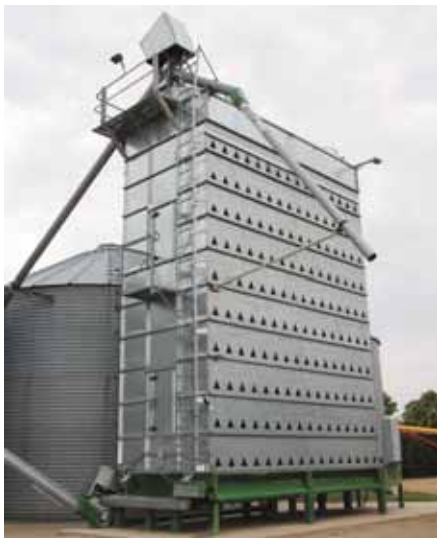
After looking at a lot of different dryers, Tim Kelly built his own continuous flow grain dryer.
