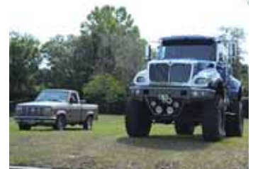
Pickup cab tops out at 10 ft. 2 in., and reaches 11 ft. 6 in. at top of exhaust pipe.
