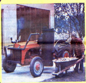
"Most any tractor can be converted to wood-gas in two days, and at a cost of about \$400," says James Bohlen, who runs his converted Ford tractor on wood chips.
