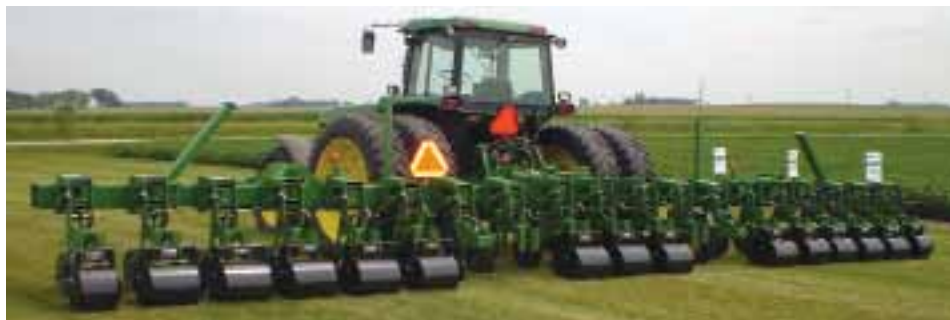
Culti-Rollers were field tested last spring on this 18-row Deere cultivator. Rollers can be filled with water or sand to add weight.
