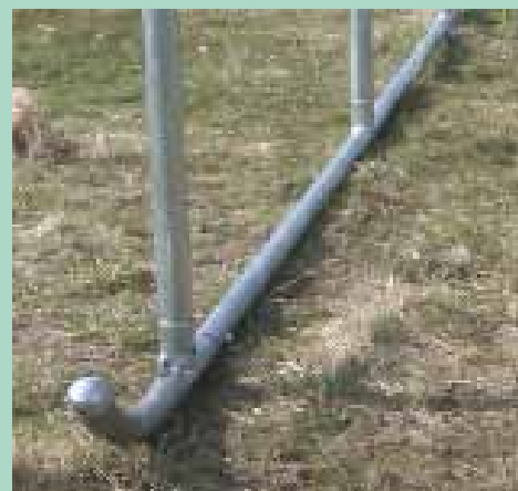
Pipe skids sleeve together for easier assembly, rounded skids help with lateral movement.
