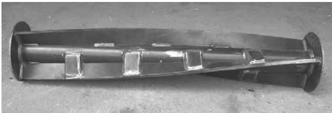
Rock beater has a spiral shape, which ensures that 70 percent of the opening in the beater is always open so crop can flow smoothly into rotor.
