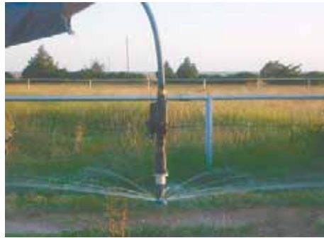
Filter fits between the hose and the regulator on center pivot drop nozzles (left). To flush out sediment you just push up a small release valve on side of filter.
