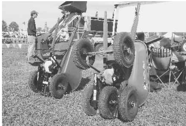
Photo shows 2-wheel-drive model, left, and 3-wheel-drive model, which is also fitted with optional rear wheel kit.
