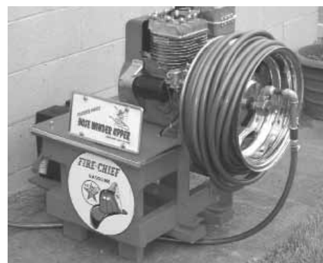
Hose winder mounts on wood frame with a 12-volt battery on back.
