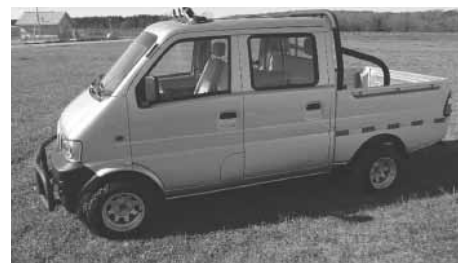
Made in China, the 4-WD, 4-door mini pickup is powered by a 4-cyl., water-cooled gas engine that gets 35 to 40 mpg.
