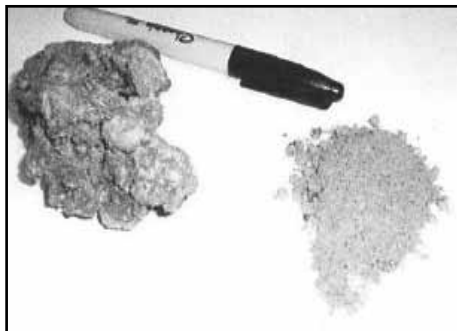
Typical clinker formed while burning hay pellets (left). Stove's ash remover reduces such clinkers into a fine powder ash (right).
