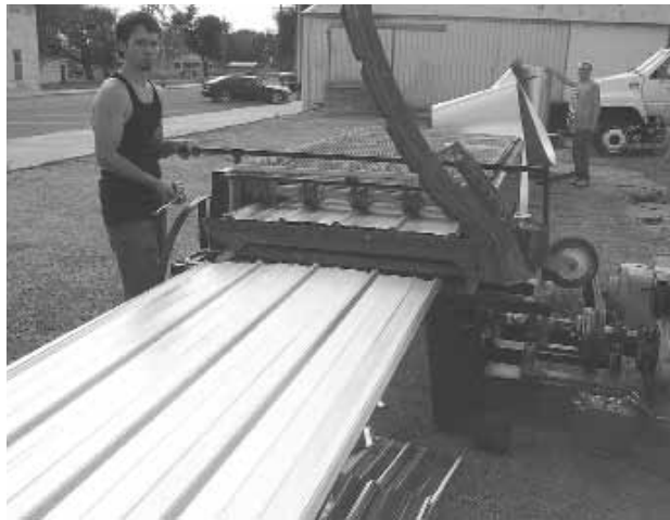
Glenn Eggmeyer rolls and sells steel roofing, and also makes and sells rolling machines.
