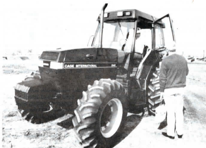
The hood tilts up and the side panels come off for easy servicing. All routine maintenance, including refueling, can be done from ground level.
