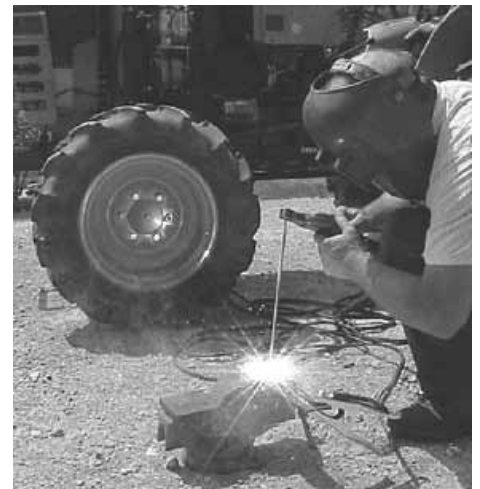
Remote controls are built into the electrode holder so you don’t need to go back and forth to your welder to readjust power.
