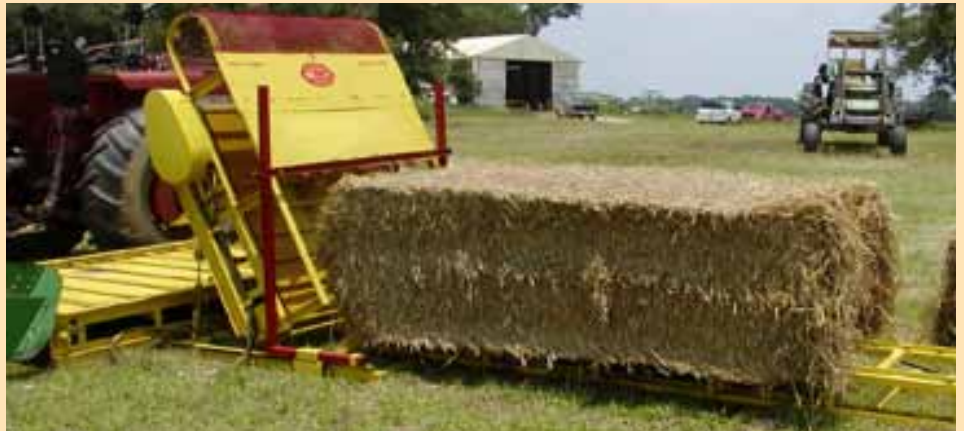
Bale feeds into separator head that pulls flakes of hay off big bale for rebaling.
