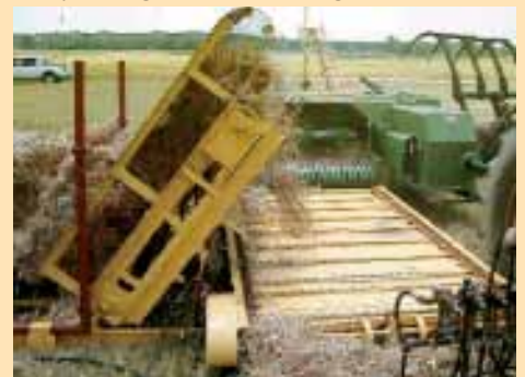
Separator head drops loose hay onto conveyor, where it feeds into small square baler. Bale elevator carries bales away for stacking.
