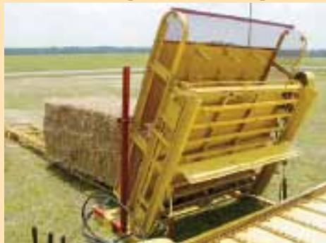
Separator head drops loose hay onto conveyor, where it feeds into small square baler. Bale elevator carries bales away for stacking.
