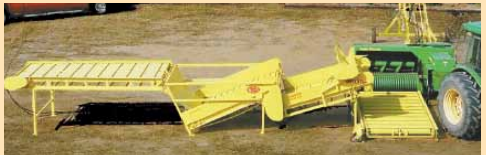
Simpson recently introduced a four piece machine. While one bale is being unrolled for rebaling, you can load another bale onto the prep-table. When the first bale is done, you just flip a lever to advance another roll into the unroller chamber. (Unit shown is four piece model.)
