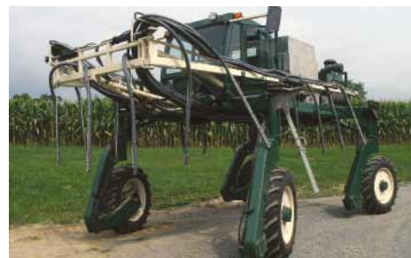
“We built it because we needed a better way to seed cover crops on our hilly ground,” says Charles Martin about his “high boy” seeder.
