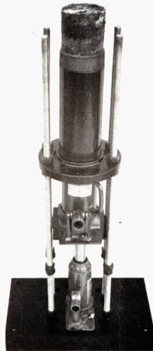
Leaves are stuffed into top of press, and the lid screwed on. Photo shows lid removed and the pressed leaf log being ejected.
