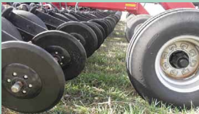
One South Dakota customer seeds 4,000 plus acres every spring. He used to replace up to 10 closing wheels per day. With the help of May Wes, he replaced all the original OEM wheels with the new May Wes UHMW solid closing wheels.
