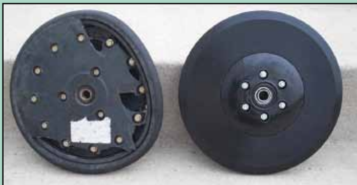
Collapsed closing wheel, left, is replaced by May Wes wheel, right.
