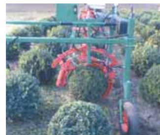
Angled blades rotate in a circle to quickly form perfect globes.
