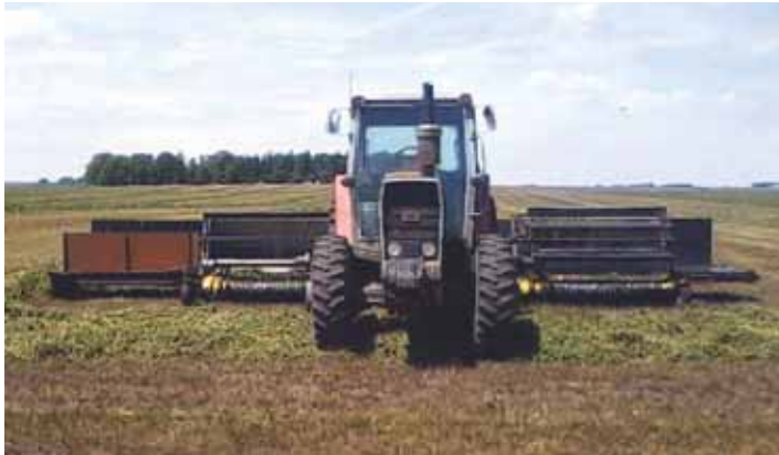
Travis Brockshus built this big 3-pt. mounted hay merger for less than a third of the cost of a commercial rig.
