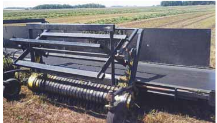
Reels installed on the rig's two 7-ft. forage heads keep hay flowing smoothly to the 32-ft. long, 4-ft. wide conveyor belt.
