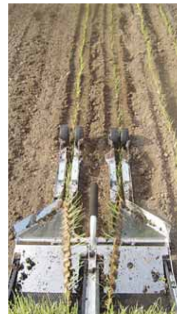
Seeds are planted into paper pots that are connected in a paper "chain" that feeds out through transplanter.
