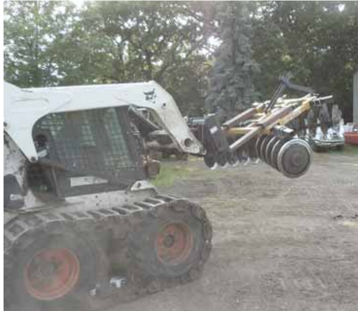
Skid steer-mounted disk lets Clyde Reilly apply more down pressure while working close to tree lines.
