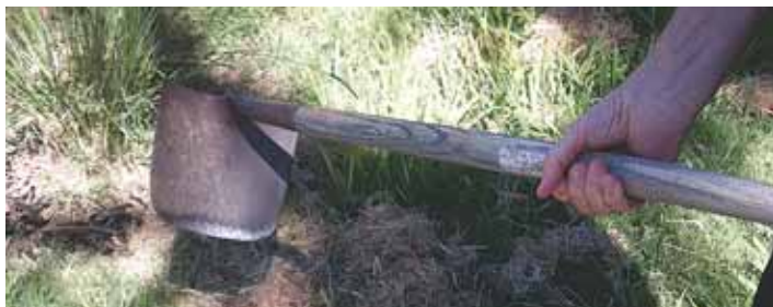
Tom Hutchinson turns worn-out shovels into heavy duty “chopping hoes”, heating the metal neck with a torch and then bending it to about an 85-degree angle.
