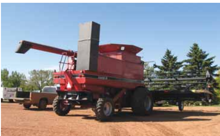
Wood 8-ft. “chimney” forms protection tunnel around combine’s air intake screen. Opening at the top allows dust-free air to enter engine.
