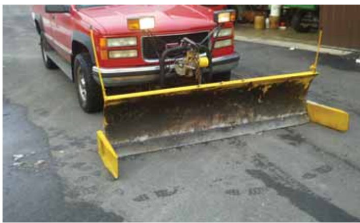
John Herren added 2-ft. wing blades to his Meyers 7-ft. snow blade, allowing the blade to move more snow.
