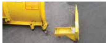
Wings drop into sockets welded to each end of snow blade.
