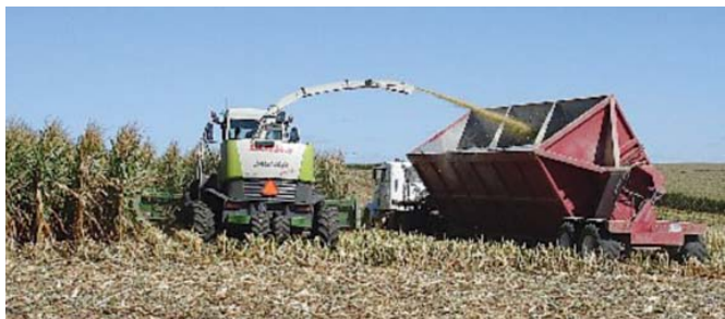
Trailer box measures 8 by 8 ft. by 34 ft. long. Hinges allow trailer driver to tip box toward chopper while loading.
