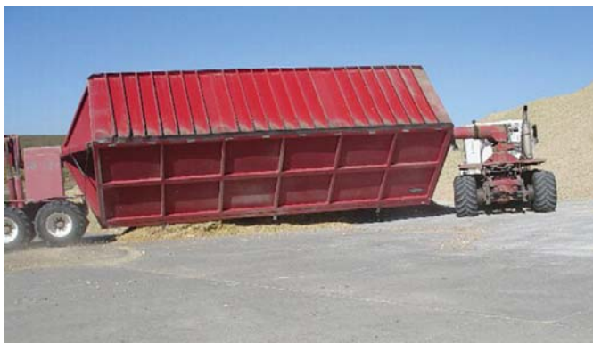
Lowell Weitzenkamp needed a big side dump trailer strong enough to handle anything from ear corn silage to composted manure. He came up with a new side dump design.
