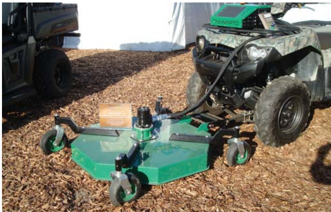
ProManPTO system for ATV's and utility vehicles uses interchangeable hydraulic motors that can be moved from one implement to another.
