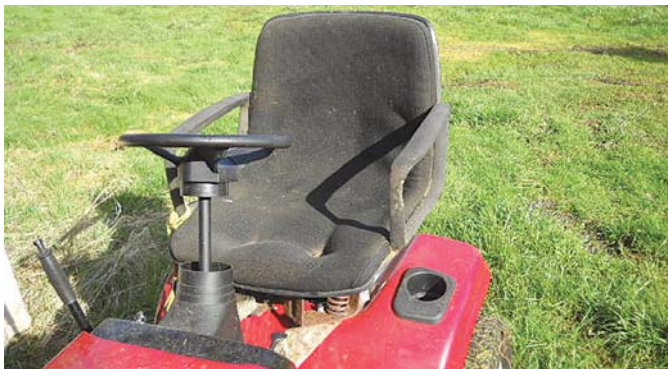
Wess Cornelius replaced the seat on his Sears riding mower with an office chair to make the ride more comfortable. He also raised the steering column 9 in.
