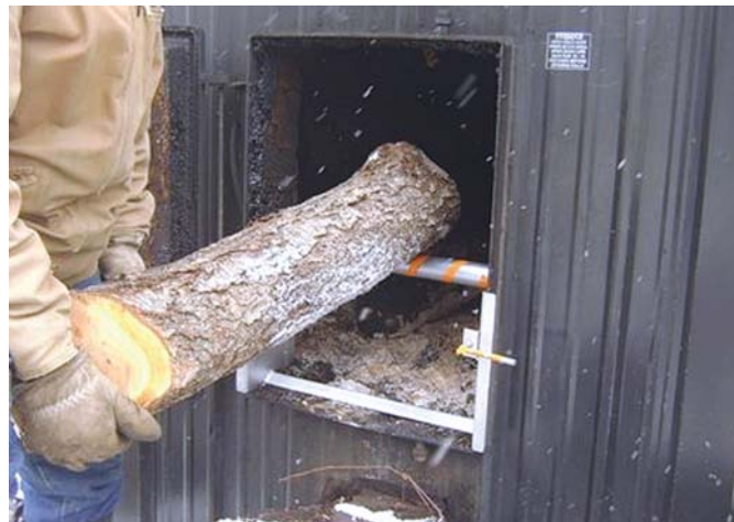
"Stove stoker" mounts on door frame and is held in place by a pair of locking handles. Steel roller on top is used to roll big logs into firebox.
