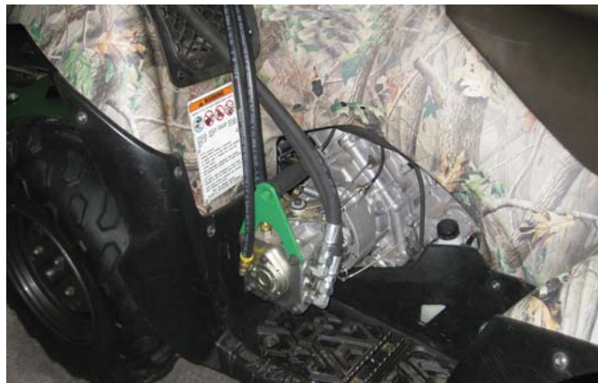
Variable displacement axial piston hydraulic pump quickly attaches to ATV or utility vehicle's engine. A twist of the handle releases pump from engine.
