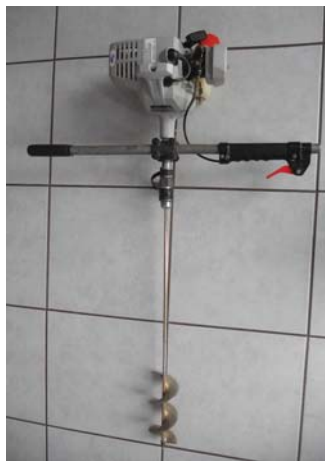
Parducci attached an ordinary bulb auger to his weed whacker. "It works fast and won't burn out," he says.
