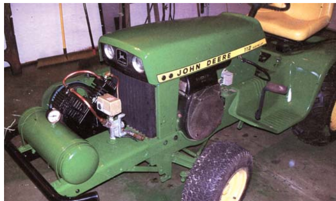
An old electric air compressor and a small portable air tank mounts on front of Sands' Deere garden tractor. Compressor is belt-driven off tractor engine.
