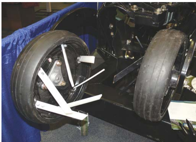
Plastic swirl strips on Dawn Strip-Till closing wheels create a swirling action that blasts soil particles against each other.
