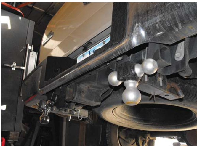
Hitch Hermit lets you store ball hitches under your rear pickup bumper, where they’re out of the way yet always accessible.
