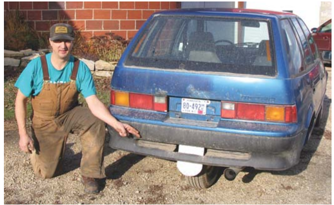
"There's nothing like it on the road," says Randy Hinzmann, who replaced the rear axle on his 1991 Geo Metro with a single center-mounted wheel.
