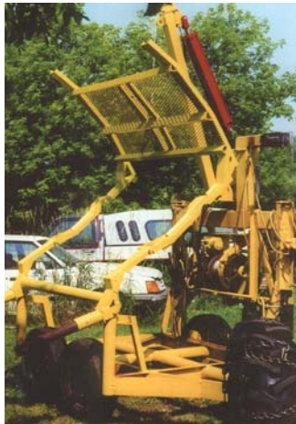
Boom is used to dump entire load at once by raising rack.
