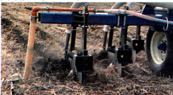
Toolbar has 20 outlets on 24-in. centers and is equipped with wavy coulters and standard knives as well as foam markers.
