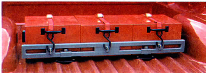
"Salt box system" consists of 3 wooden boxes positioned side by side across pickup bed directly over the rear axle. Boxes are secured with steel plates to bed.
