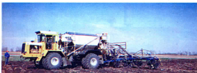
Deep bander is equipped with an 8-ton Tyler airflow box that's turned backward.
