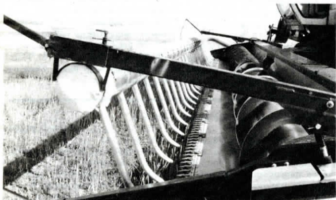
The operator of this A-C Gleaner combine, equipped with a 30 in. Airway system, harvested 10 bu. per acre wheat at 9 mph.
