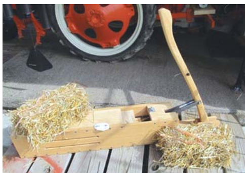
All-wood mini baler makes 6 by 6 by 12-in. bales. A 3-ft. long axe handle compresses straw inside a long wooden box, which forms the body of the baler.
