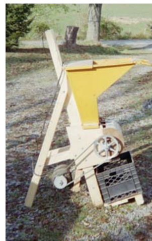
Walnut huller uses an electric motor to belt-drive a wooden drum inside a metal cover. Both the hulls and nuts fall into an old milk crate.
