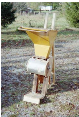
Walnut huller uses an electric motor to belt-drive a wooden drum inside a metal cover. Both the hulls and nuts fall into an old milk crate.
